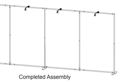
1) Assemble frame together in numerical order. 2) Apply pillowcase graphic over assembled frame, then zip closed.
